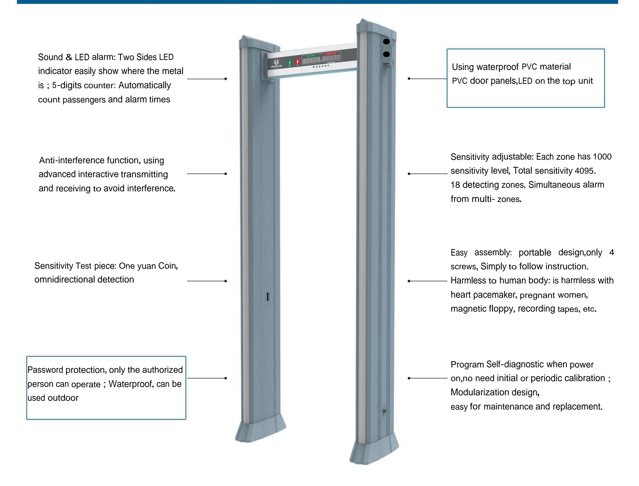
Walk Through Metal Detector is mainly used for routine security checking. When the passengers carry metal content over preset parameters value, the detector will automatically alarm, meanwhile side LED lights will accurately indicate the alarm location. It greatly helps security guards faster and easier to find out the prohibited metal objects, such as guns, knives, keys...etc.
