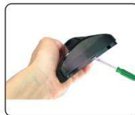
Use a screwdriver to open the back cover of the product
