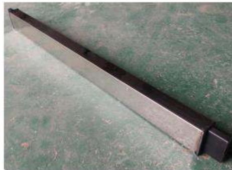
Name: bottom rail Material: SUS201# Spec.: 75*45 squire tube color: nature color T: 0.75mm
