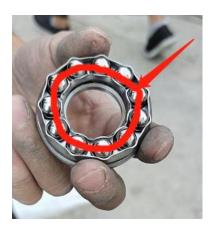
1.2 In addition, the floor of the base must be horizontal and if the rotating rod is not concentric, the bearing will be damaged very soon.
