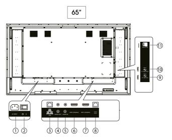
(1) AC IN - (2) Main Power Switch - (3) LAN - (4) Audio OUT - (5) Audio IN - (6) HDMI2 IN ⑦ HDMI1 IN - ⑧ RS232 - ⑨ USB Port 2 - ⑩ USB Port 1 - ⑴ Micro SD
