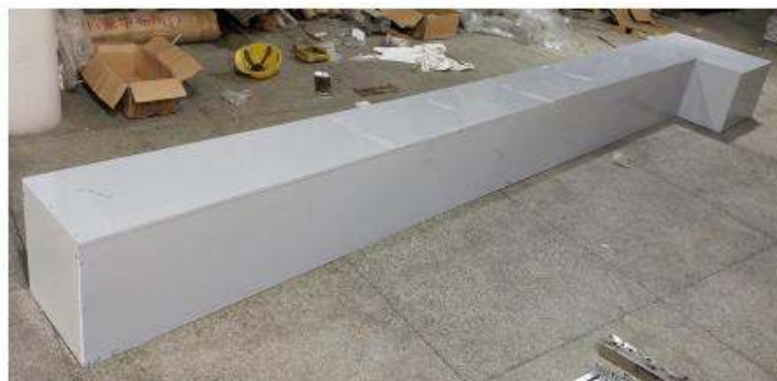
Name: cover box Material: SUS201# Total lenght=8100mm The zinc square pipe is used as the support frame, and the cover plate is buckled on the galvanized pipe. It is a split type. When the customer is installed on site, it needs to be assembled in two butt joints.
